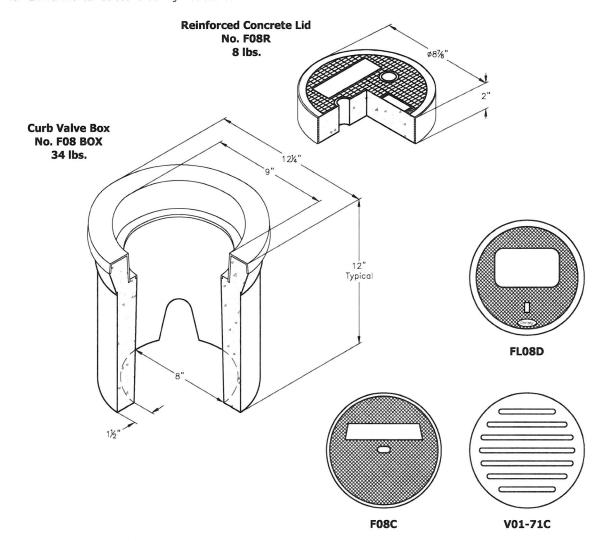
A high density reinforced concrete box with non-settling shoulders positioned to maintain grade and facilitate back filling. Approximate dimensions and weight shown.
