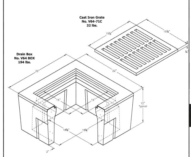
This concrete drain box has a cast in galvanized frame and is specfically engineered for drainage in medium areas such as parking lots, school grounds, walkways, ects. Its design permits final grading material to "lock in" and finish clean. Knock—outs accommodate up to 8" O.D. pipe. Approximate dimensions and weight shown. ADA approved grates available upon request.
